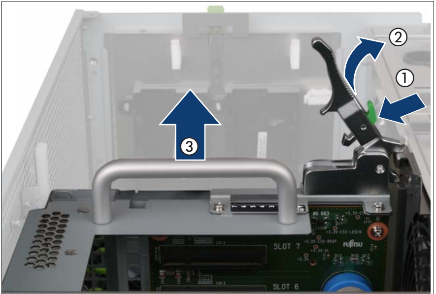
Figure 148: Removing the PCI Riser
